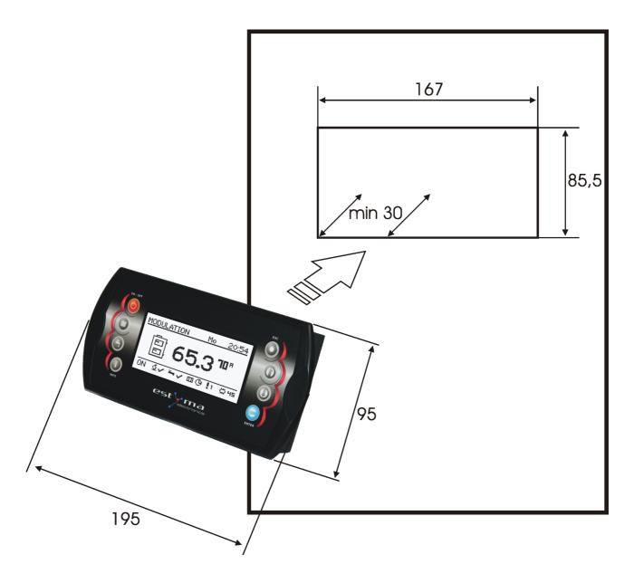
After placing the panel in the hole, always install the mounting frame.
