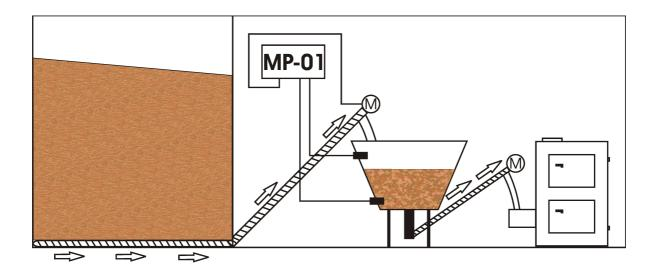
The sensors must be placed inside the tank boiler according to the descriptions. Bottom sensor must be mounted at the bottom of the tank, the upper sensor at the top.
