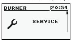
In the list, you can locate the position **Lambda control**, which switches on **YES**. It is also possible working with switched off Lambda control mode. Then Lambda oxygen sensor module will be responsible only for displaying the measurements.
